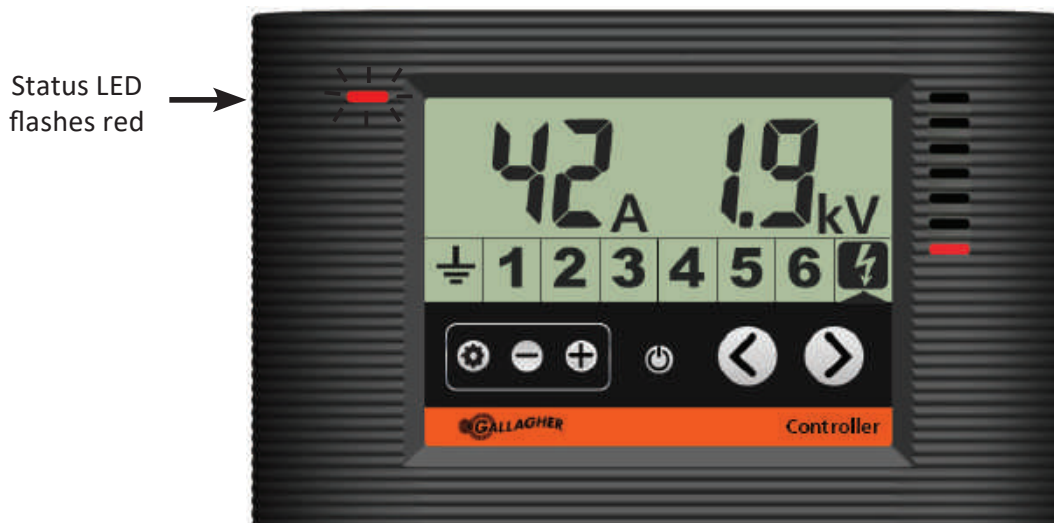
Controller showing the energizer in output alarm
