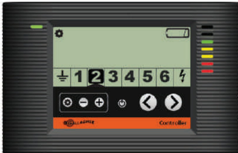
Controller showing zone 2 with a low battery
