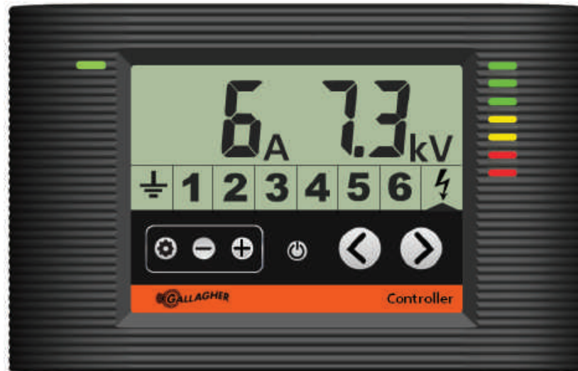
Controller showing the energizer operating normally
