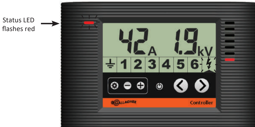
Controller showing the energizer in current alarm
